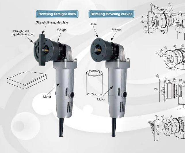
For corners (R), straight lines and curves **One-touch Beveller**  •Firmly grasp the body of the beveller, place the base plate on the work object and work slowly with the tip touching the object.
